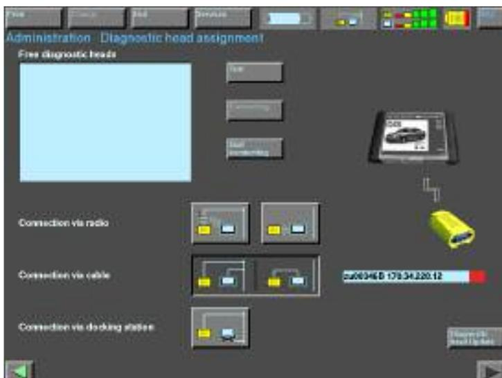
The diagnostic head is communicating with the diagnostic machine.
