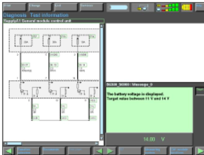
The test plan utilizes the MFK 1 leads as an input for the measurement. By pressing start, the measurement is automatically taken from these leads.
