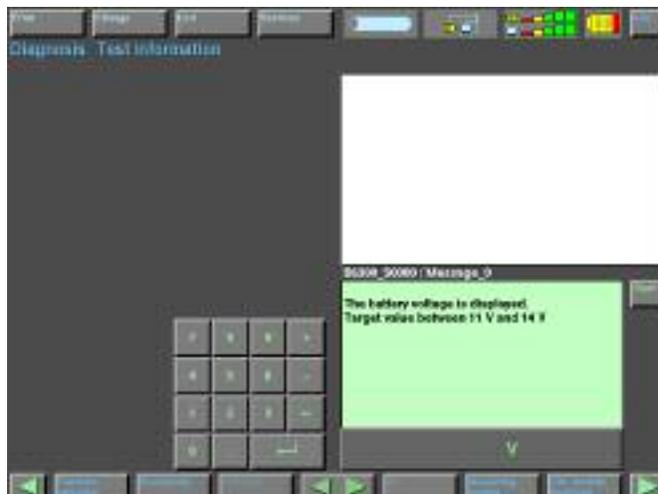
If you are using a DVOM for measuring the values in place of the MFK leads, you can enter the measured values into the system and follow the test plan as follows:
