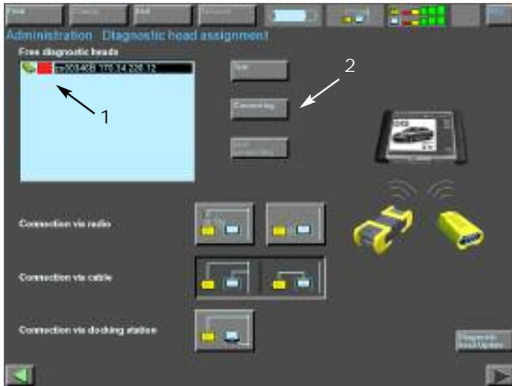
Select the free diagnostic head desired (1), and press "Connecting" (2).
