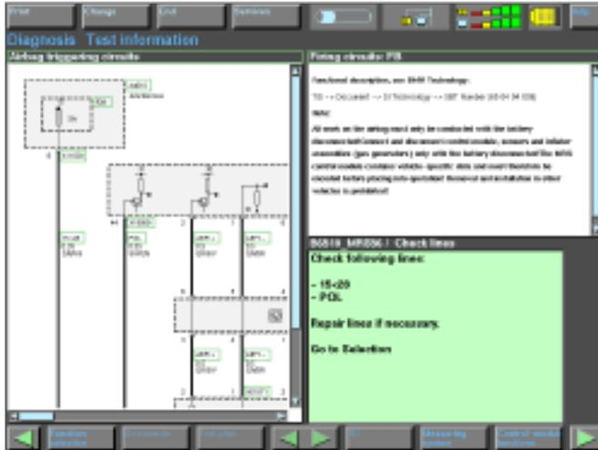
The diagnostic program in the tester has measuring capabilities an integral part of the the test procedure. It displays automatically when needed by the test plan.
